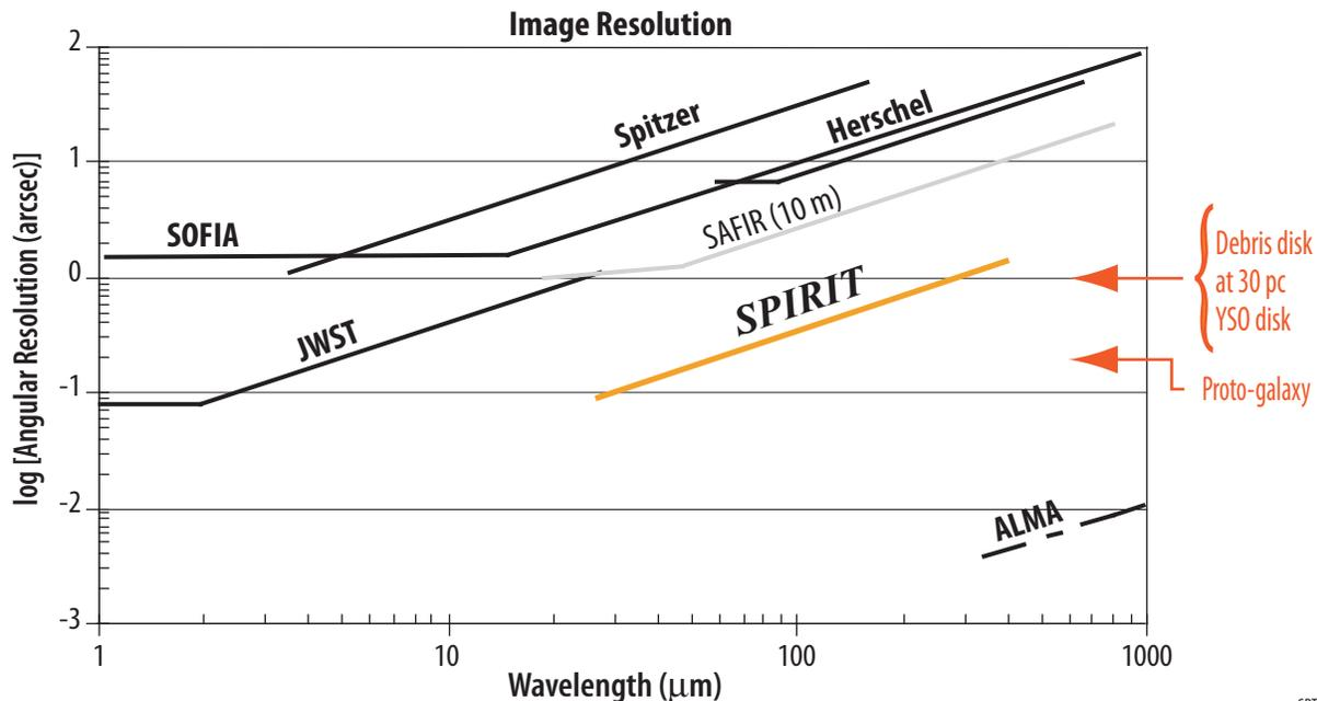
**Figure 4:** SPiRiT will deliver one hundred times better angular resolution than Spitzer, and resolution comparable to that of JWST, but at ten times longer wavelengths, where protoplanetary disks, debris disks, and some galaxies emit most of their light.
