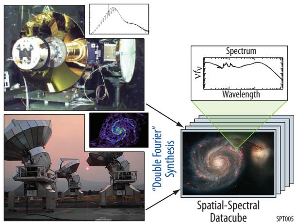
**Figure 5:** SPiRiT combines the capabilities of an imaging interferometer with those of a Fourier Transform Spectrometer to produce spatial-spectral data cubes.
