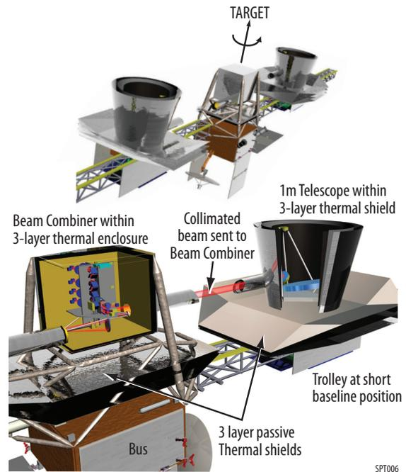
**Figure 6:** Major components of the SPiRiT observatory are two movable afocal off-axis telescopes and a single beam-combining instrument.
