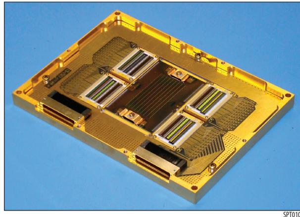
**Figure 10:** This 8 x 16 array of close-packed TES bolometers saw first light at IRAM in 2007.<sup>[83]</sup> This was the first fielded array with backshort-under-grid architecture, a technology developed to enable and mature versatile, space-qualifiable kilopixel TES arrays with NIST large-format SQUID multiplexers.
