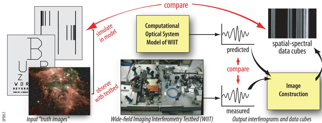
**Figure 12:** WIIT, a laboratory testbed functionally equivalent to SPIRIT, and a high-fidelity model of the testbed, are giving us practical experience with the wide-field double-Fourier interferometric technique to be used on SPIRIT.
