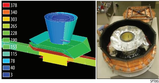
**Figure 7:** (Left) Heat loads and cryocooler requirements were based on a 106-node thermal model. (Right) Subscale cryo-thermal testing in a LHe shroud validated the model.
