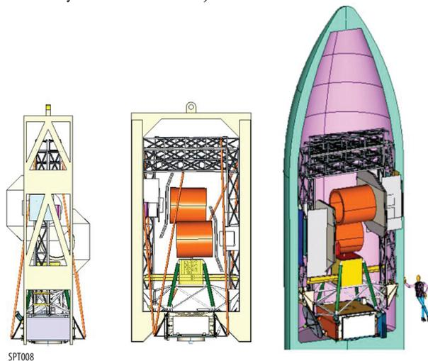
**Figure 8:** SPIRIT and its expendable launch support structure (left, two views), when stowed for launch, are 8.7 m tall and fit into an EELV 5 m medium-length fairing dynamic envelope.
