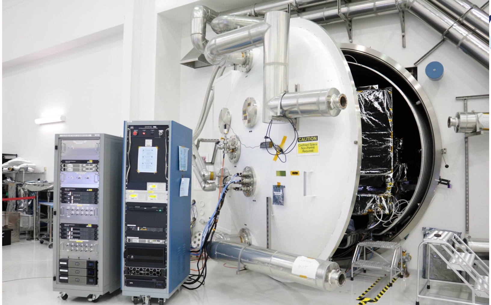
Now: limited functional tests before closing the chamber door
