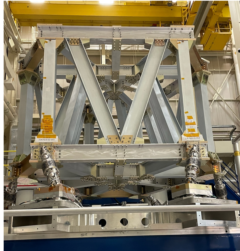
6 LLVIS struts supporting payload mass simulator on vibration table
