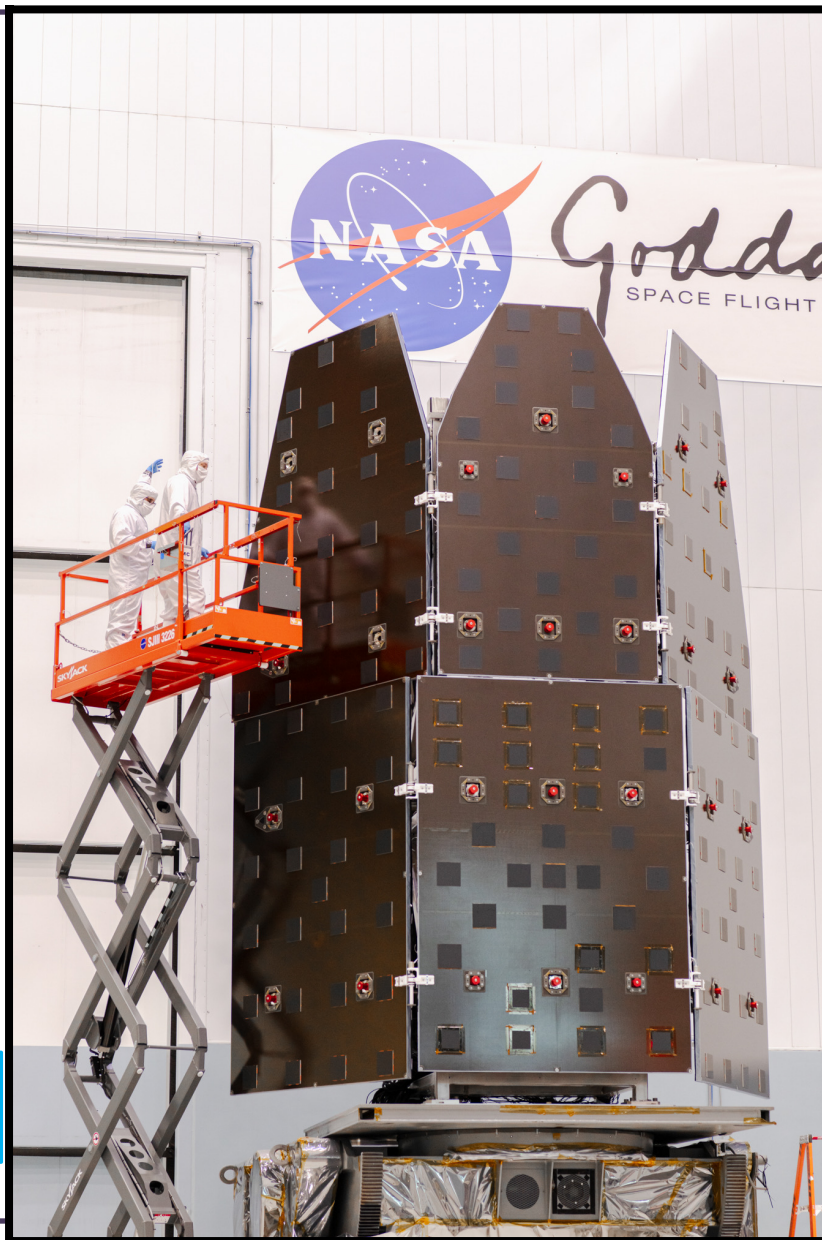
Deployment Testing of Surrogate Solar Array / Sunshield (SASS) panels
