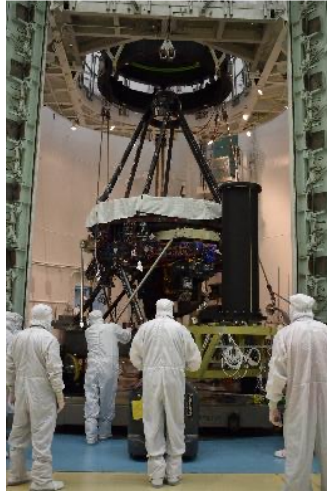
IOA being moved into Chamber IIIB for Alignment
