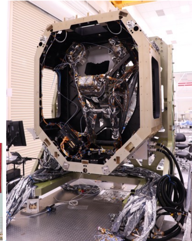
Alignment Compensation Mechanism (ACM), Optical Bench, Enclosure, Latches, and Element Wheel Assembly have been integrated
