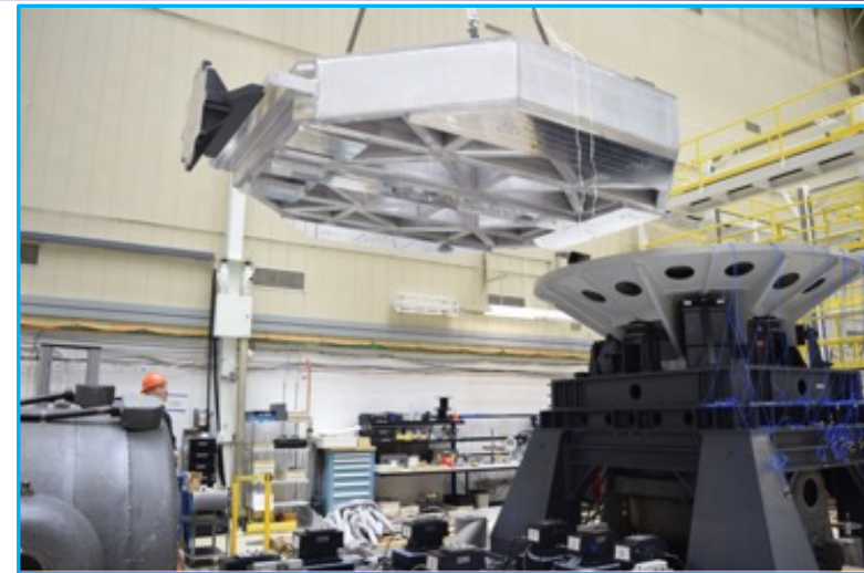
(OTA) Lateral Vibe weldment flying over to the head expander
