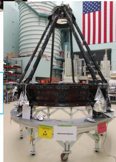
Forward Structure Assembly complete and ready for the next level of integration
