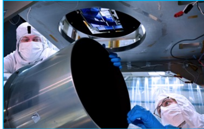
(WFI) Flight Focal Plane Assembly pre-vibration thermal/vacuum testing completed
