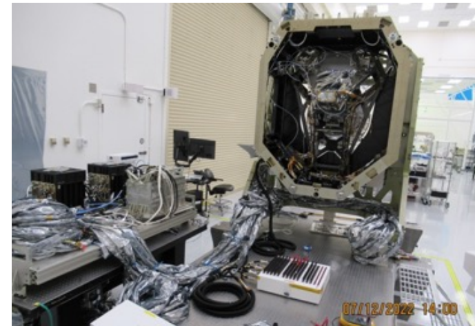
(WFI) Cold Module and Warm Electronics have been integrated and tested at Ball
