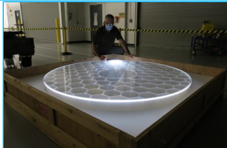
(OTA) Optical Large Aperture Flat System (OLAFS) mirror ready for Mounted Mirror Assembly (MMA) integration
