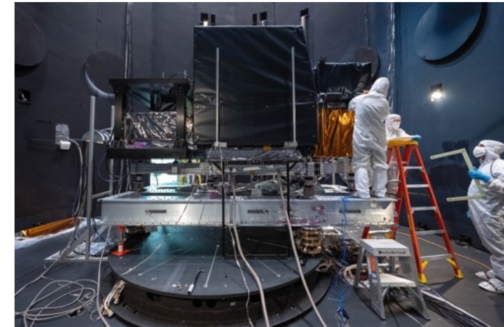
Stimulus of Ray Cones (SORC) is in thermal/vacuum testing in the Space Environment Simulator chamber
