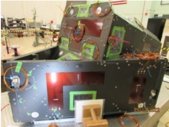
Aft Optics Structure (AOS) Thermal-electric work in progress
