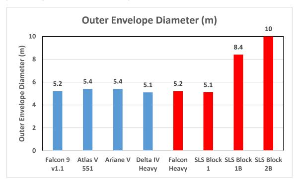
Figure 2 - Launch fairing diameters for a variety of current and future launch vehicles. Existing vehicles are in blue, ones in development are in red. These outer diameters correspond to the exterior physical extent of the fairing. Inner diameters are developed through coupled loads analyses with particular payloads and are roughly 0.5 to 1 m smaller. All these fairing diameters are representative values subject to evolution of existing vehicles and refinement of designs in development.
