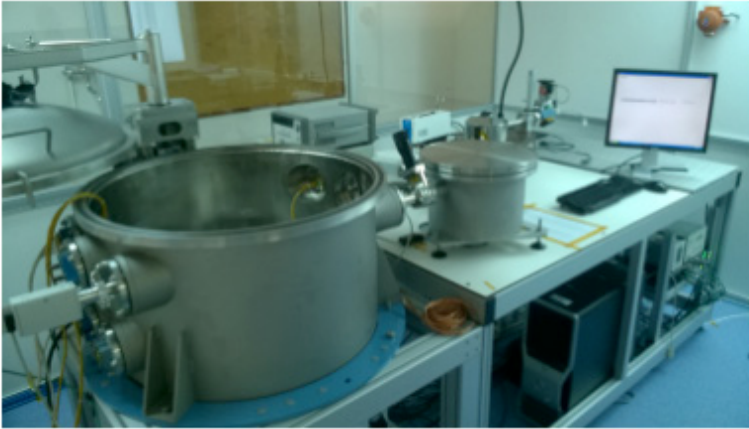
Figure H-9. Left: Bench and vacuum chamber at LATMOS. Right: Experiment built at LESIA for the FUV polarimeter, currently placed in the vacuum chamber.
