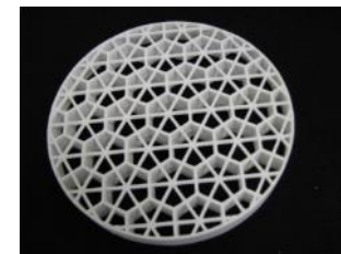
Innovative mirror designs enabled by 3D printing
