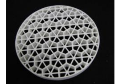
3D Printed Architecture for Lightweight Mirrors
