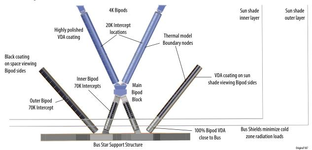
Figure C-6: Spacecraft bus bi-pods/strut and 4.5 K Bipods have heat intercepts at 20 and 70K and VDA or Black paint coatings located to minimize heat flow to the Cryogenic Payload Module.
