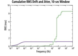
**Figure 2-34:** (left) Drift and jitter performance during inertial pointing complies with requirements under reasonable worst-case assumptions. Wavefront sensor noise drives drift performance, while cryocooler disturbances drive jitter performance.
