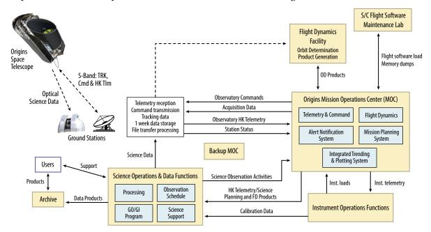
**Figure 2-50:** The *Origins* Ground System is similar to those employed for other large NASA missions and includes the use of optical communication technology advances to downlink the mission's large science data volume.
