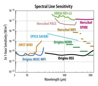
**Figure D-19:** The 5 $\sigma$  1-hour line sensitivity of the Origins /MISC WFI (R=300) module.
