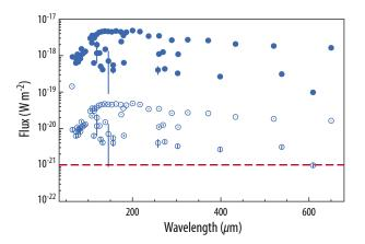
**Figure A-14:** 50-650 µm line fluxes for BHR71. Fluxes are scaled to the luminosity of L1014 at a distance of 200 pc (filled blue circles) and at 2000 pc (open blue circles). The *Origins*/OSS detection threshold (dashed red line) assumes the line emission is unresolved.
