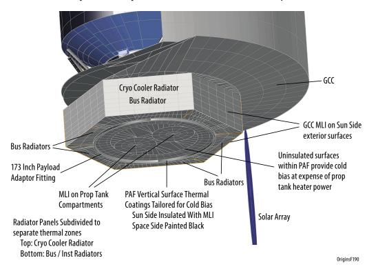
**Figure C-9:** The thermal aspects of the spacecraft bus are designed to minimize CPM interface temperatures while accommodating over 4kW electronics dissipated power.
