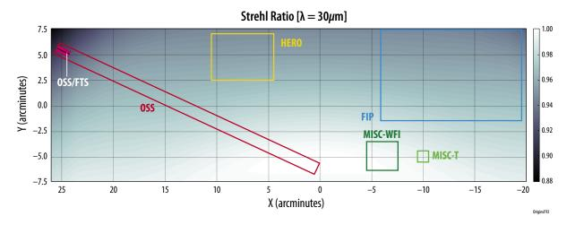
**Figure D-2:** An evaluation of the upscoped *Origins'* RMS wavefront error as a function of FOV shows that the performance requirement (less than 0.07λ) is met across each instruments FOV. Note that the colorbar is set such that light corresponds to better optical performance and dark to poorer optical performance.
