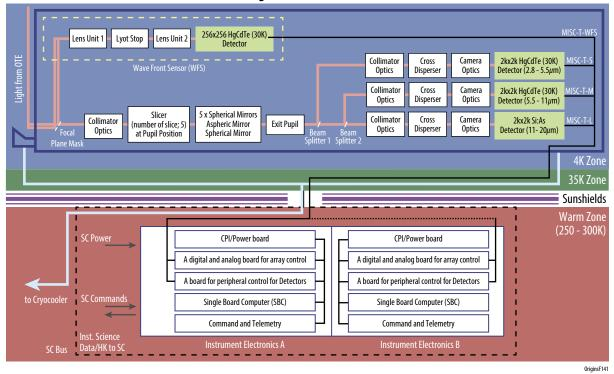
Figure 3-14: The MISC-T block diagram showing the optical paths, detector focal planes, electronics, and temperature regimes.
