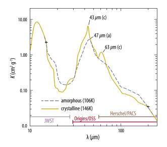
**Figure A-10:** *Origins* can detect the presence of water-ice, as well as study the thermal history of grain mantles by observations of the 43, 47, and 63 µm features. The plot shows the water-ice opacities (McClure et al., 2015). Characteristic wavelengths of the amorphous (dashed line) and crystalline (solid line) ice emission maxima are noted with a and c, respectively.
