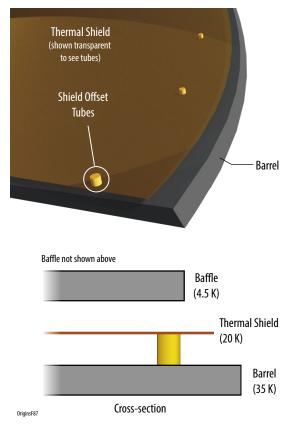
**Figure 2-19:** The Thermal Shield is offset from the Barrel to provide an effective radiative shield. The shield is fastened to thin-walled Vespel® tubes mounted to the inside of the Barrel.
