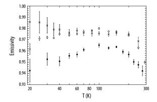
**Figure C-4:** Emissivity measurements made for BIRB show it is very black at low temperatures. The 0.65 kg/m<sup>2</sup> sample (X) used for JWST was also used in this model. This application of BIRB will be used for *Origins*.
