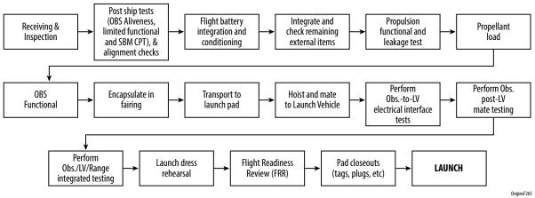
Figure C-76: Origins Top Level Flow for Launch Site Operations
