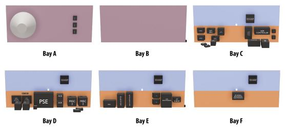
**Figure C-28:** Bay A Components, showing the Communication Antenna Dish's enclosure and three diplexers. Bay C-F Components; the upper (blue) section of the side panel is the cryocooler heatsink and contains embedded heatpipes. Components mounted to the Bottom Close-out panel appear to be floating.
