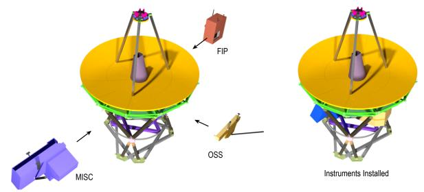
Figure C-19: Instrument ground support equipment is used to carry each instrument into area under the PMBSS.
