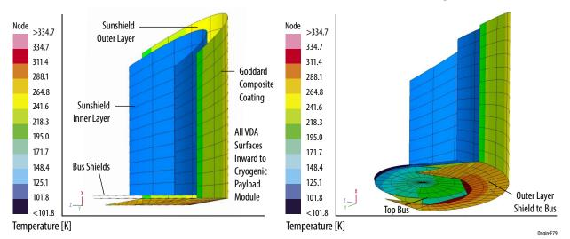
Figure 2-11: The Outer Sunshield with GCC maintains room temperature or lower for all FoR over nearly all of its surface.
