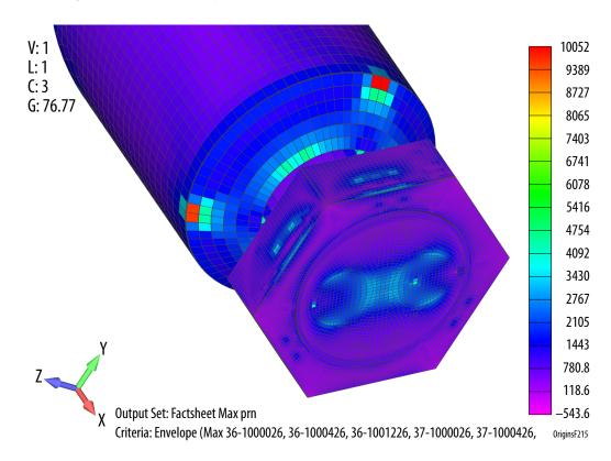
Figure C-34: The highest stressed aluminum honeycomb facesheet component is located at the interface of the Barrel cylindrical side panel and conic bottom panel. Colors denote stress levels in PSI.
