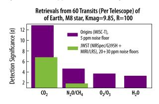
**Figure 1-55:** Detection significance comparison between JWST and *Origins*. Assuming noise floors of 20 and 30 ppm for NIRSpec/GRISM and MIRI/LRS, respectively, JWST will only be sensitive to  $CO_2$  at >3.60. With a 5- ppm noise floor, *Origins* will be sensitive to  $CO_2$  and the biosignature pair  $O_3$ +N<sub>2</sub>O. Figure courtesy Kevin Stevenson (STScI).
