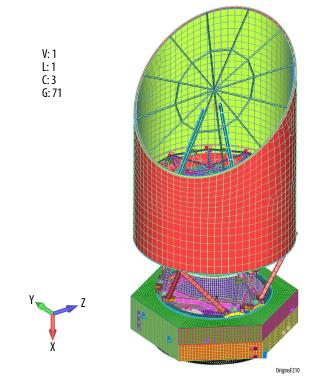
**Figure C-29:** The *Origins* observatory finite element model shows a very detailed design for an accurate first-cut analysis. Colors denote different components.
