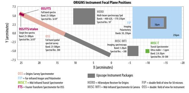
**Figure 2-2:** The *Origins* Space Telescope focal plane showing all the instruments studied and the result of the descope exercise. Those items shown in grey were descoped and two (HERO & MISC-WFI) of these are described as possible upscopes in Appendix D.
