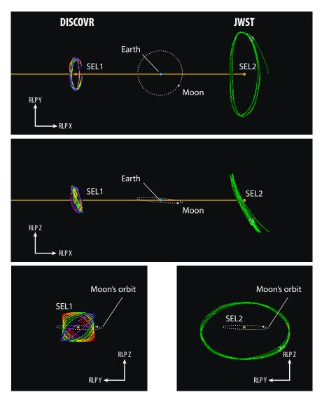
**Figure C-77:** JWST and DSCOVR orbits are shown in the XY, XZ, and YZ Rotating Libration Point Frame show examples of the various orbits (shown to scale) that can be achieved at the Libration Points.
