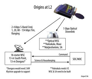
Figure 2-38: Origins Communication System Consists of Optical Downlink of Science Data and S-Band for Command & Telemetry
