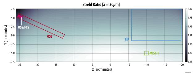
**Figure 2-25:** An evaluation of the baseline *Origins* Strehl ratio as a function of FOV shows that the performance requirement (greater than 0.8 Strehl ratio) is met across each instruments FOV. Note that the colorbar is set such that light corresponds to better optical performance and dark to poorer optical performance.
