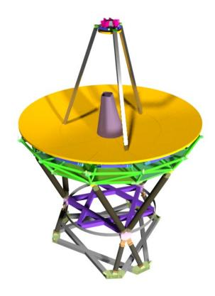
**Figure C-18:** Each Primary Mirror Segment Assembly is installed, then the Tripod, then the Secondary Mirror, and finally the Aft Optics Structure.
