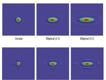
**Figure C-50:** PSFs for circular and elliptical aperture shapes showing that asymmetry in the in the aperture shape leads to undesired asymmetry in the PSF. The circular aperture was chosen for *Origins*.
