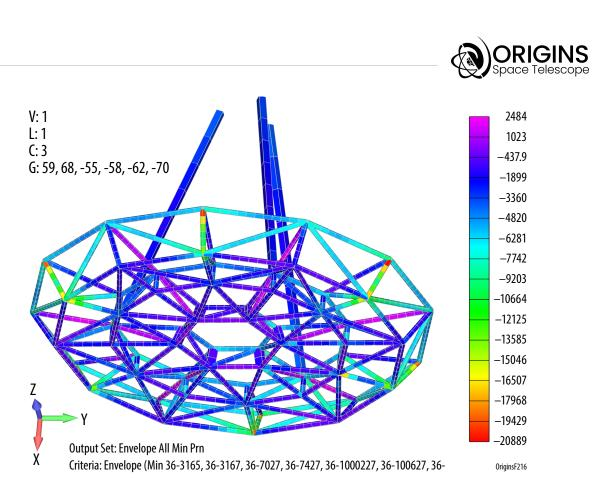
Figure C-35: The highest stressed beryllium tube component located at the top end of a vertical tube. Colors denote stress levels in PSI.
