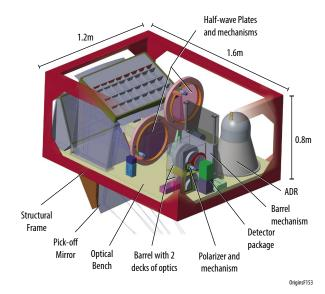
**Figure 3-26:** The FIP mechanical structure and components. The labels point out individual components described in the text.
