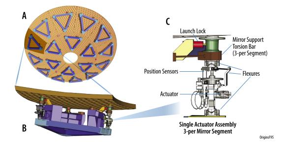
**Figure 2-27:** The (A) *Origins* Primary Mirror Segment Assembly showing a (B) mirror segment and (C) actuating mechanism is based on proven designs. Each segment uses three JWST actuators with flexures to ensure kinematic, reproducible motion.
