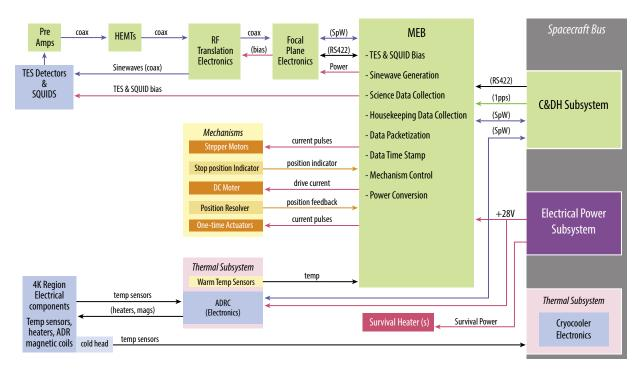
Figure 3-31: This FIP Block diagram shows how the instrument is controlled.
