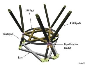
**Figure 2-17:** The *Origins* Bipod Support Subassembly base supports three sets of Bus Bipods, which support the 35-K Deck. The bottoms of the 4.5 K Bipods are attached to the 35 K Deck.
