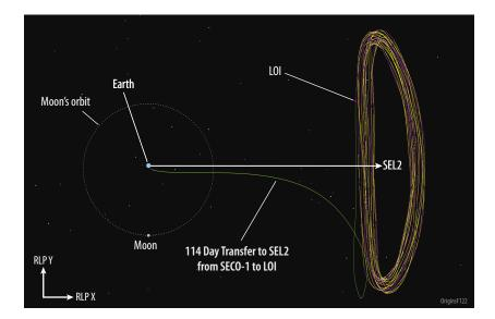
**Figure C-81:** *Origins* transfers to SEL2 over 114 days before executing a LOI maneuver to insert itself into the mission orbit.
