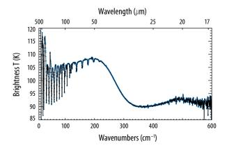
**Figure A-17:** Far-IR spectrum of Saturn, as measured by *Cassini*/ CIRS, showing the rotational lines at the longest wavelengths and the smooth collision-induced continuum that allows temperature, windshear, aerosol, para-H<sub>2</sub> and helium sounding. Comparable, repeatable, and spatially-resolved measurements are desired across the discs of each giant planet (from Fletcher et al., 2015).
