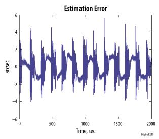
**Figure C-59:** Pointing knowledge during survey operations complies with the 2-arcsec RMS requirement at all times. The square-wave pattern apparent in the plot is due to the raster scan survey pointing profile.
