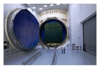
**Figure C-68:** Chamber A at JSC will be used to perform CPM cryogenic testing.
