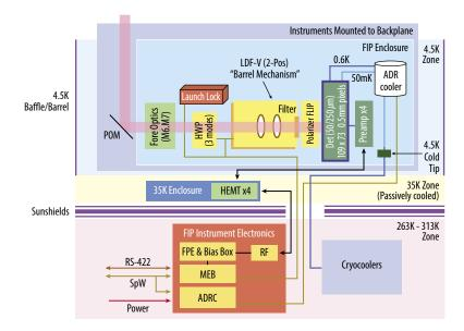
**Figure 3-25:** FIP has a simple design with one detector selectable by filter to 50 or 250 µm. This Functional Block Diagram of FIP shows how the power dissipation in the cold 4.5 K section is minimized by placing the readout electronics in the warm part of the observatory.
