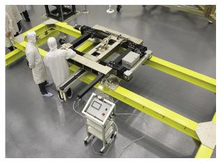
Figure 2-45: Variable Center of Gravity Mechanism
