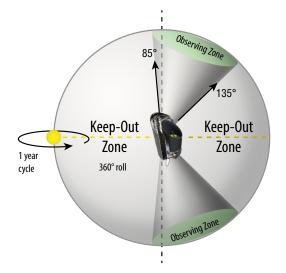
**Figure 2-51:** The mission's FoR allows *Origins* to observe within  $+85^{\circ}$  to  $+150^{\circ}$  (note error in Figure caption) off- pitch off the sun line, yaw 360° around the sun line, and roll  $\pm 5^{\circ}$ .
