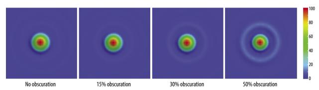
Figure C-49: Comparison of PSFs for increasing values of linear obscuration for an on-axis telescope
