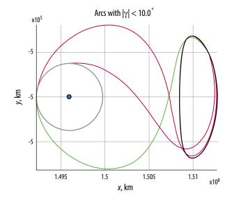
**Figure 2-54:** Stable and Unstable Manifold Transfer between SEL2 to Lunar Orbit, Angle <10°
