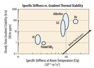
**Figure C-54:** Steady state gradient stability plotted against specific stiffness at room temperature shows beryllium (Be), AlBeMet<sup>®</sup>, and SiC as the best performers.
