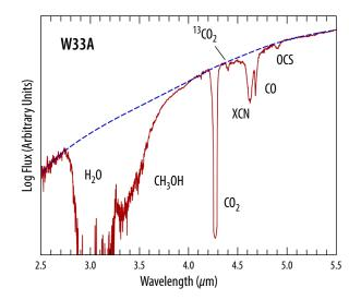
**Figure A-11:** Near infrared spectrum of the star forming region W33A obtained by ISO (Sloan et al., 2003). The blue dashed curve shows the dust spectrum expected without ice, while the red spectrum shows changes to the dust spectrum caused by the buildup of various ices on the grain surface. The composition of the ices between 2.5 and 5 µm is noted above.
