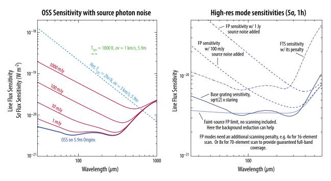
Figure 3-10: Sensitivity of OSS for bright sources (left) and in the high-resolution modes (right). The etalon (FP) curves refer to the required scanning time to be incorporated
