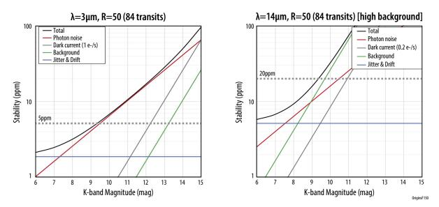
**Figure 3-23:** The current best estimate of the spectro-photometric stability achieved by MISC-T. Left: 3  $\mu$ m with R=50 is below 5 ppm for stars brighter than magnitude 9.5. Right: 14  $\mu$ m with R=50 (high Zodical background case; Wright 1998) is below 20 ppm for stars brighter than magnitude 9.3. See the text for further explanations.
