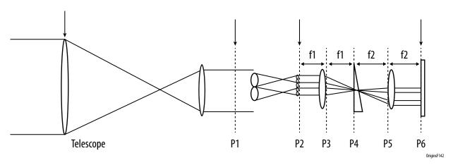
**Figure 3-15:** A schematic diagram of the densified pupil concept. Light from the telescope is collimated into a conjugate pupil plane P1. This plane is divided into sub-apertures (two of which are shown in this figure) and the light is then further focused by lenslets or mirrors into an array of optical paths, each with its own spectral dispersion path, in a conventional spectrometer configuration (P2-P5) with the spectra then imaged onto the detector (P6).
