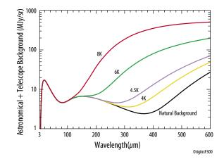
**Figure 4-9:** Increasing the *Origins* telescope temperature even slightly relative to 4.5 K pushes the telescope into a regime in which it dominates natural astronomical background photon noise and severely compromises *Origins* science.
