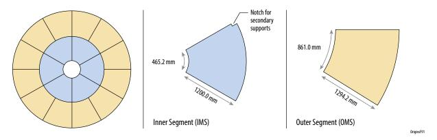
**Figure 2-23:** The twelve *Origins* primary mirror outer segments are identical. The inner segments are of one design, with three of the six mirrored to accommodate a notch for the secondary mirror struts.
