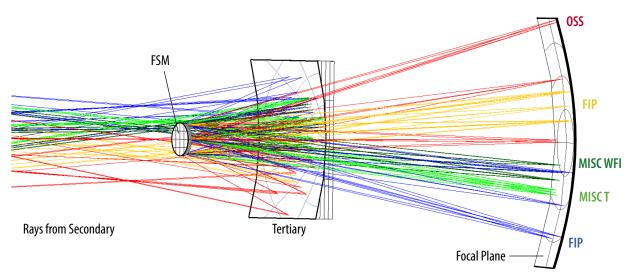
**Figure D-1:** CODEV<sup>®</sup> layout showing rays for each of the upscoped instruments passing through the telescope onto the image surface. As compared to the baseline design, this includes the addition of the MISC imager channel, the HERO instrument, and increased FOVs for both FIP and OSS.
