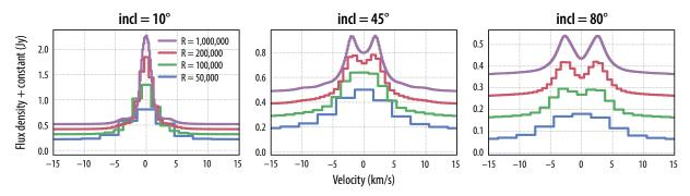
**Figure E-4:** The 179.5 µm water ground-state line simulated for different inclinations and resolving powers shows that the double peak at intermediate inclinations is separated only at resolving powers of at least R=200,000. Origins resolves these lines and is capable of exploiting the kinematic information.
