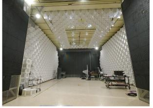
**Figure C-73:** Large EMC Shielded Enclosure
