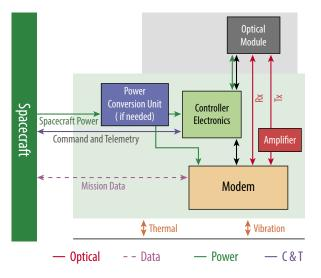
Figure C-60: Flight Optical Terminal Block Diagram
