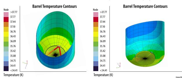
**Figure 2-12:** The Barrel temperature contours show that the barrel temperature remains below 36 K and nearly isothermal in the worst case attitude (150° pitch) over nearly all of its surface.
