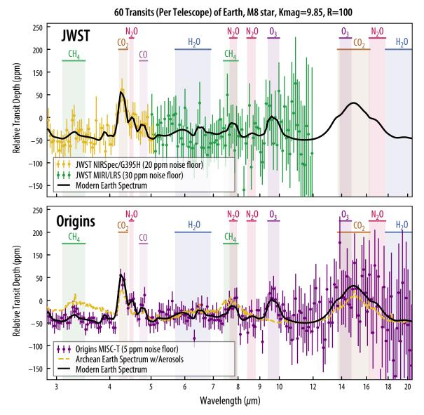
**Figure 1-54:** With its broad wavelength coverage and anticipated noise floor of 5 ppm, *Origins/MISC-T* is designed to detect key habitability indicators and biosignature gases. These plots show simulated transmission spectra for a TRAPPIST-1e-like planet with an Earth-like composition (60 transits, R = 100), comparing JWST and *Origins* measurements based on current best estimates for their respective instrument noise floors (20 – 30 ppm for JWST; 5 ppm for *Origins*).
