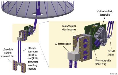
Figure D-8: The mechanics and ray trace of HERO's focal plane unit show a very compact design.
