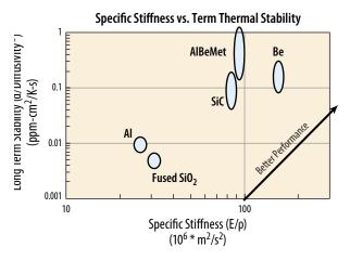
**Figure C-55:** Long-term stability (thermal diffusivity/CTE) plotted against specific stiffness at room temperature shows beryllium (Be), AlBeMet<sup>®</sup>, and SiC as the best performers.
