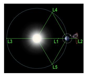
**Figure 2-47:** Our Solar System has five Sun-Earth Libration Points where a spacecraft can be maintained in a relatively-stable environment for performing observations.
