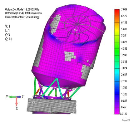
Figure C-30: Primary lateral frequency mode shape is driven by the barrel of the observatory. Colors denote strain energy levels.
