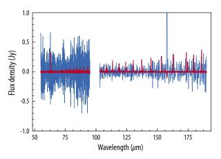
**Figure A-13:** Modeled far-IR spectrum (red) of VeLLO L1014. The model is scaled from the emission line spectrum of BHR71 Herschel-PACS data (BHR71 – 13.5 L<sub>☉</sub>; L1014 – 0.1 L<sub>☉</sub>, both at 200 pc; Green et al., 2013; Yang et al., 2017, Yang et al., 2018), compared with the actual PACS spectrum of L1014 (blue). The strong [CII] emission line at 157 µm is contaminated by background in the PACS spectrum.
