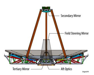
**Figure 2-31:** Aft Optics Structure mounts to the PMBSS and contains the tertiary mirror and Field Steering Mirror.
