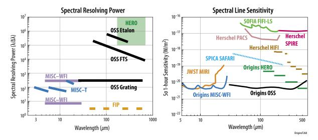
**Figure D-3:** Origins upscope option ideally complements the Origins baseline configuration by adding the capability of very high spectral resolution observations at high line sensitivity (HERO), by adding an mid-IR MISC imager, adding the 100 and 250 micron windows of FIPS and by increasing the mapping speed of OSS.
