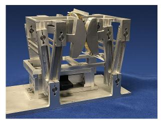
Figure 3-7: Flex type mechanism for use with the OSS FTS. This mechanism is free of friction, can be operated in any orientation and has a stroke of 10 mm. For OSS this would be scaled up by a factor of 3.
