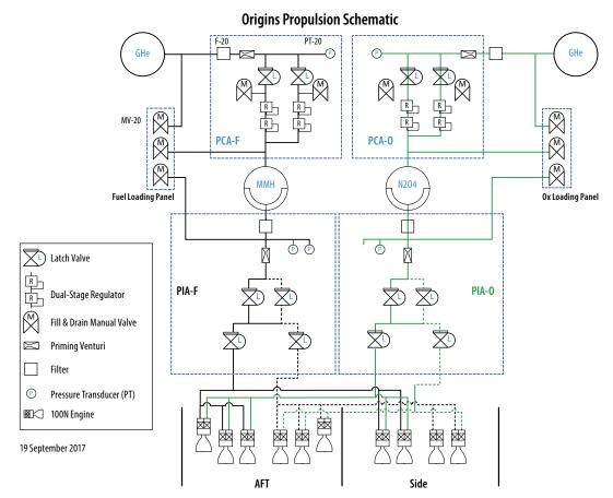
Figure 2-35: The Origins regulated bipropellant propulsion system is based on heritage designs from Solar Dynamics Observatory and Europa Clipper.
