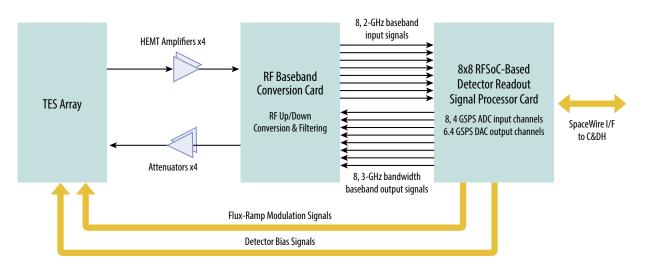
Figure 3-28: Detector readout scheme for FIP: FIP and RFSoC samples and processes signals simultaneously.
