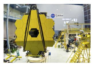
**Figure 2-43:** The JWST telescope was assembled in the Spacecraft Systems Development and Integration Facility at NASA.
