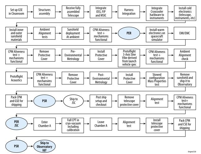
**Figure C-69:** (Above) The CPM I&T flow shows a simple path to achieve a fully-tested and -verified CPM.
