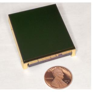
**Figure 3-24:** Long-wavelength HgCdTe detectors have been developed for NASA's NEOCam mission.
