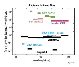
**Figure 3-32:** A comparison of photometric survey times for a number of space-based FIR instruments. Note that Origins/FIP will be the fastest mapping far-IR survey instrument ever flown in space.
