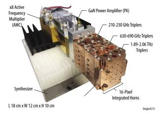
**Figure D-7:** Compact multi-pixel electronically tunable LO systems have been demonstrated to 1.9 THz.
