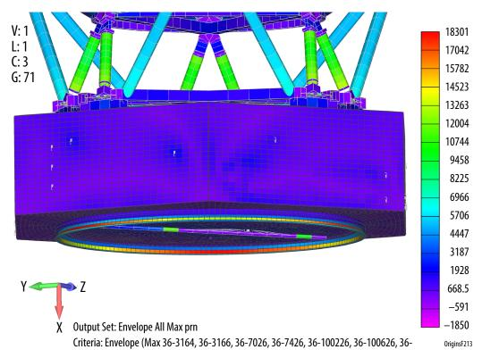
Figure C-32: The highest stressed aluminum component is the Lower Interface Ring that interfaces with the Payload Adapter Fitting. Colors denote stress levels in Pounds per Square Inch (PSI).
