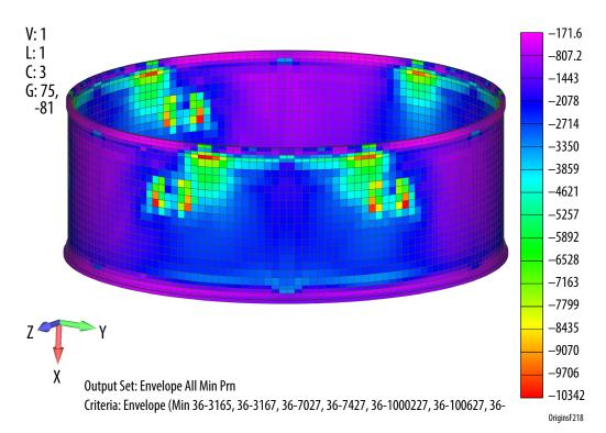
**Figure C-37:** The highest stressed M55J fiber composite component is shown along the side of the tube and indicated by red elements. Colors represent stress levels (PSI).
