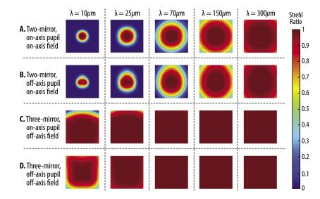
**Figure C-48:** Comparison of Strehl ratio as a function of FOV for four different telescope configurations. In each case the performance is evaluated over the same 1° x 1° full FOV.
