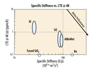
**Figure C-53:** The coefficient of thermal expansion (CTE) at 4.5 K plotted against specific stiffness at room temperature shows beryllium (Be) is the best performer, followed by AlBeMet<sup>®</sup>, SiC, fused silica, and aluminum (Al).
