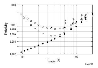
**Figure C-3:** The open circles are data from the work of Tuttle, et al. (2104, 2008). The emissivity of VDA-coated Kapton has been measured accurately from 10 K to room temperature. *Origins* uses these data to accurately account for temperature dependent emissivity.
