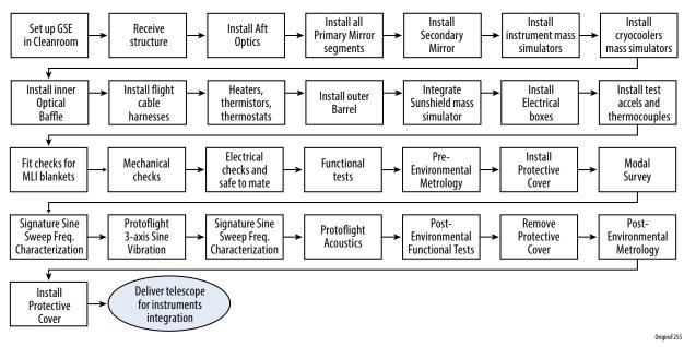
Figure C-66: Telescope I&T Summary Flow
