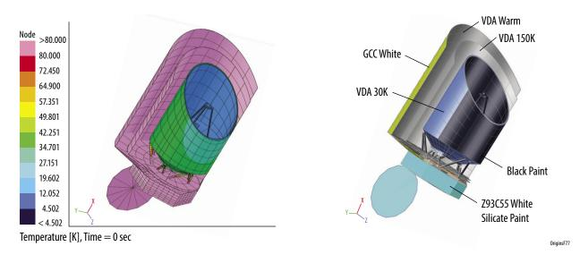
**Figure 2-9:** A Spitzer-like architecture with staged cooling, a two layer sunshield, a deep space radiator, and cryocoolers delivers the required thermal performance with a relatively simple-to-model design.
