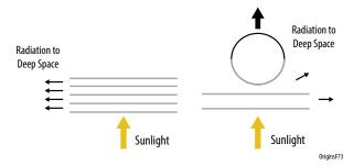
**Figure 2-4:** A two-layer sunshield plus radiator can achieve the same radiative temperature as a five layer sunshield.
