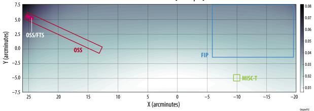
**Figure 2-24:** An evaluation of the baseline *Origins*' RMS wavefront error as a function of FOV shows that the performance requirement (less than 0.07λ) is met across each instruments FOV. Note that the colorbar is set such that light corresponds to better optical performance and dark to poorer optical performance.
