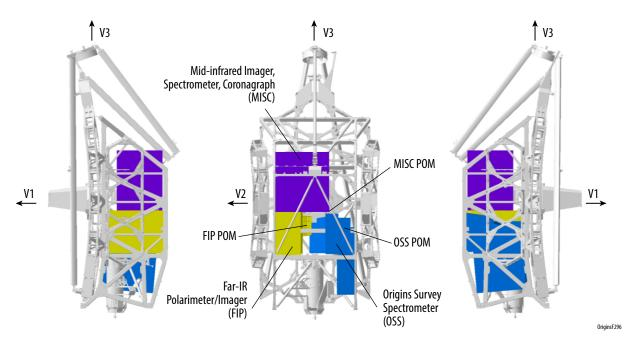
Figure F-7: Origins instruments packaged in the ISIM and IEC volumes within the JWST structure.
