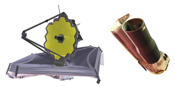
Figure 2-3: The Origins architecture is more like Spitzer (right) than JWST (left).
