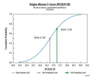
**Figure 4-7:** The CEMA-generated *Origins* Mission-Level S-Curve gives the likelihood that the cost will not exceed a particular value. Cost estimates at 50% CL and 70% CL in Base Year 2020 dollars are shown.
