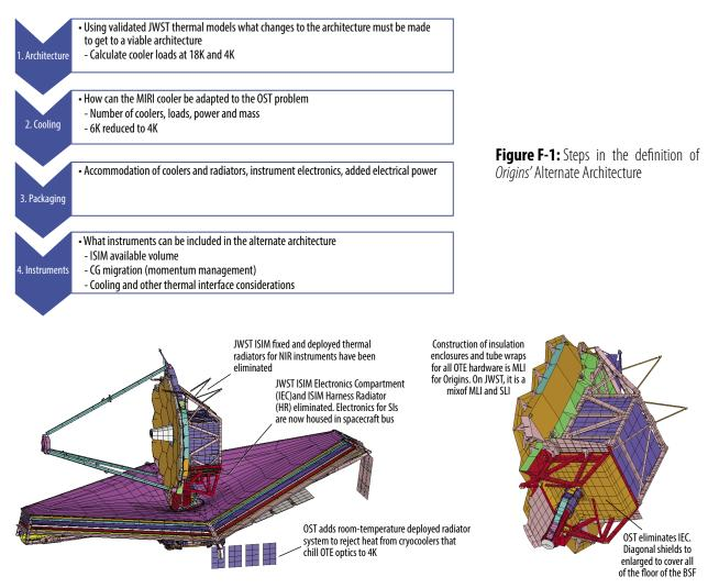
Figure F-2: View of the JWST derived Origins Alternate Architecture
