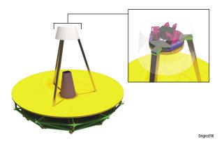
**Figure 2-30:** The Secondary Mirror Subassembly mounts on the end of a tripod connected directly to the PMBSS.
