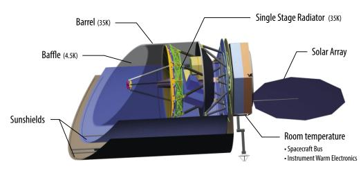
**Figure 2-5:** Origins temperature zones are designed to maximize cryo-cooling efficiency while ensuring a 4.5 K environment for the telescope and instruments. The instruments are housed in the 4.5 K zone beneath the primary mirror. The 35 K radiator is more clearly shown in Figure 2-9.
