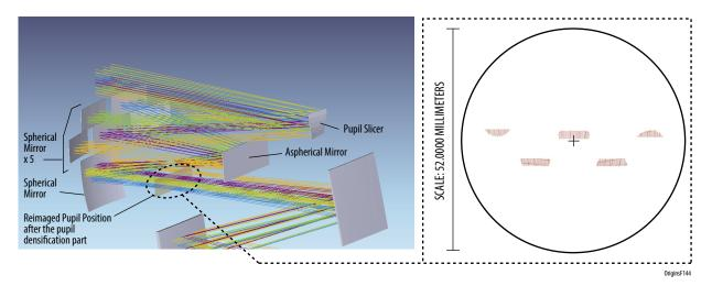
Figure 3-17: The telescope pupil is reimaged and sliced as shown at left, with the slices separated as shown in the image on the right.
