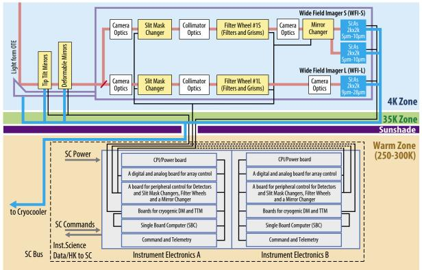
Figure D-16: The MISC WFI block diagram indicates the second module that was added to the upscoped MISC instrument.
