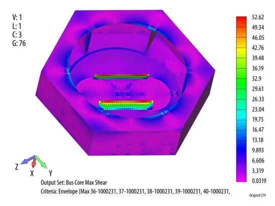
Figure C-38: The highest stressed aluminum hex core component are the fuel tank skirt supports. Colors indicate shear stress levels (PSI).
