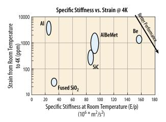
**Figure C-56:** Strain from room temperature down to 4 K against specific stiffness at room temperature shows tradeoffs between be-ryllium (Be), AlBeMet<sup>®</sup>, SiC and fused silica with aluminum (AI) as the lowest performer.
