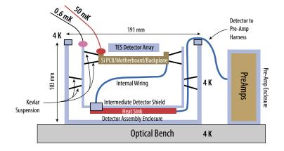
**Figure 3-30:** The FIP Focal Plane Array is cooled to 0.05 K and suspended within a 0.7 K enclosure, providing thermal shielding from the 4.5K stage. The Kevlar suspension, which is common to most instruments with low temperature detectors, provides for excellent stiffness while having a very low heat conductivity.
