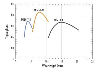
**Figure 3-22:** The throughput as a function of wavelength used for MISC-T performance calculations.
