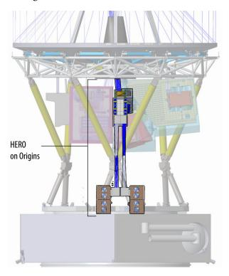
**Figure D-10:** HERO is a relatively small instrument that fits easily into the spacecraft. To minimize the cryogenic heat load the reference signal (Local Oscillator) is located in the spacecraft bus and optically linked to the cold unit (blue ray traces).
