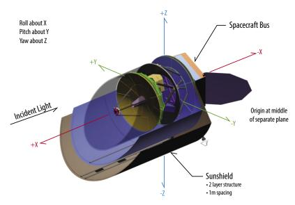
**Figure 2-7:** Origins cut-away view showing the observatory coordinate system. The Spacecraft Bus Module is toward the back right in this view and the Cryogenic Payload Module is everything front and left of that including the telescope barrel and sunshields. The Origins coordinate system uses +X as the boresight and -Z as the direction to the Sun when the pitch angle is 90 degrees and the roll is 0 degrees.
