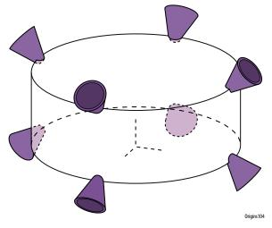
**Figure 2-36:** Current best estimate (CBE) engine locations on the *Origins* spacecraft bus provide delta-V and three- axis control.
