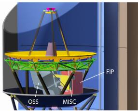
**Figure 2-32:** Each instrument under the backplane of the primary mirror assembly. This location is effective for maintaining the instruments (and mirror) at 4.5 K in the cryo-payload module (CPM, Section 2.3).
