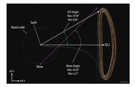
**Figure C-78:** *Origins'* transfer trajectory and mission orbit for 10 years shown in the RLP XY Frame with corresponding LEV and Moon Angles meets current requirements
