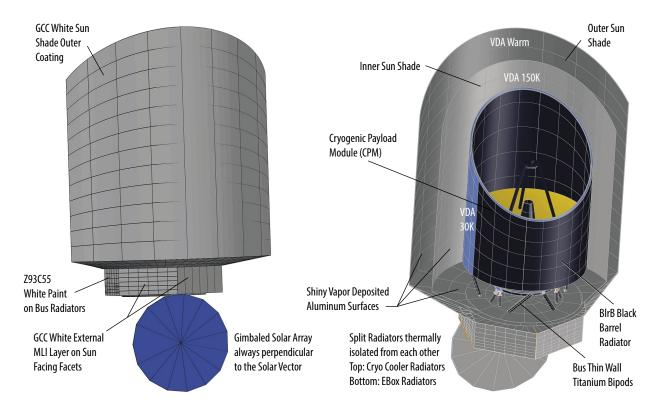
Figure C-1: End to End Thermal modeling of the entire observatory for the full attitude range at SEL2 establishes thermal design feasibility.
