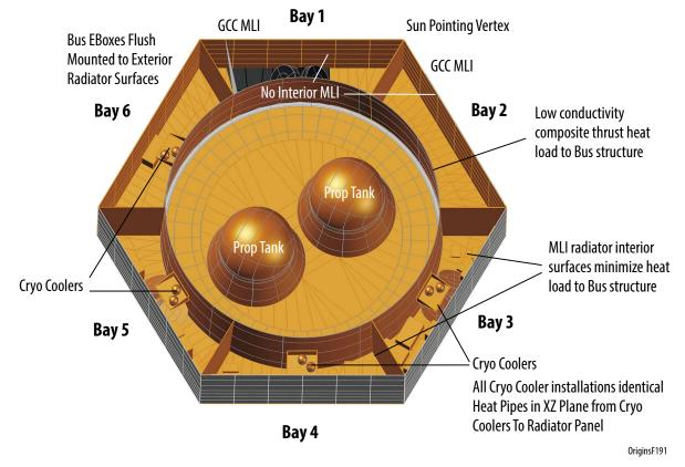
Figure C-10: The spacecraft bus thermal model interior view shows how the various heat loads are localized to each radiator panel.
