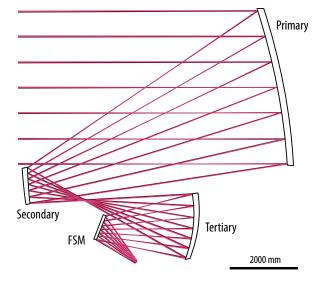
**Figure C-52:** Resulting optical design utilizing a spherical primary mirror. The design concept was not further pursued for *Origins* due to poor optical performance.
