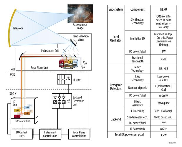
**Figure D-6:** The HERO is the first heterodyne array receiver designed for space. The schematic diagram shows a relatively simple design that covers the widest frequency coverage and the highest sensitivity of any heterodyne receiver. HERO uses sensitive state-of-the-art components with low power consumption and weight.
