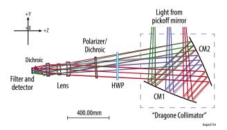
**Figure 3-27:** The FIP optical system minimizes the number of optical components. This configuration shows the layout for a polarization measurement because the HWP is in the beam.
