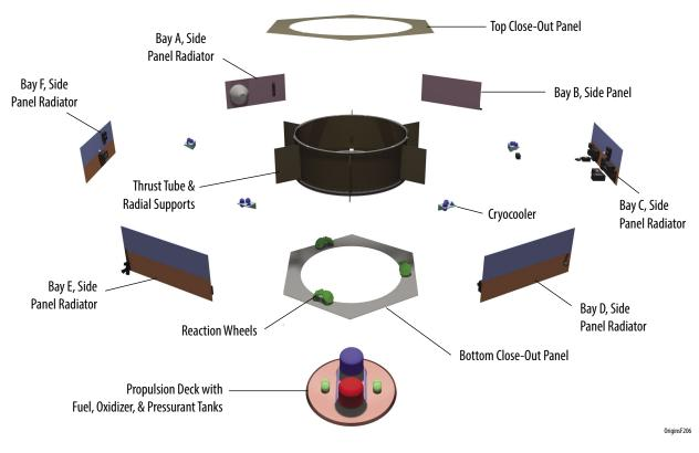
Figure C-25: The Origins Spacecraft Bus, Exploded View
