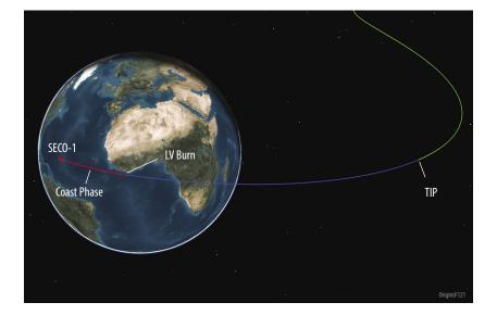
**Figure C-80:** *Origins* will then coast along its parking orbit until a state is reached where the Launch Vehicle will perform a large maneuver that will place *Origins* on the correct outbound trajectory to SEL2.
