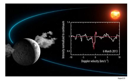
**Figure D-5:** Water is ubiquitous in our solar system. Detection of water vapour around the dwarf planet Ceres. The narrow 557 GHz H<sub>2</sub>O line was detected with HIFI in October 2012 and 2013 (Kueppers et al, 2014, Nature).
