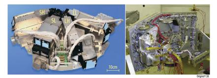
**Figure 3-11:** Previous missions provide heritage for the basic approach of the OSS elements. The bolted aluminum OSS grating spectrometer uses the same approach as the Spitzer infrared spectrograph from Houck et al., 2004. Its four wideband modules are shown at left. The Fourier-transform module path-folding approach and mechanism use the same approach as in the Herschel SPIRE instrument shown at right (Griffin et al., 2010).
