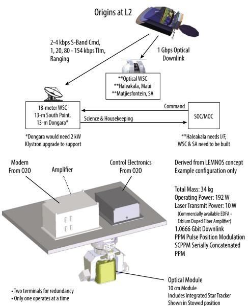
Figure C-58: The Origins optical communication system is fully redundant.
