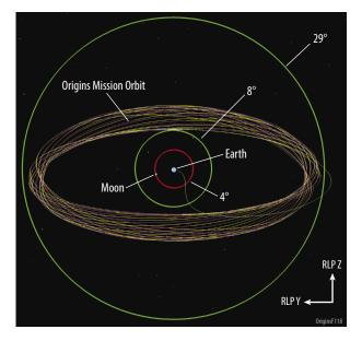
**Figure 2-49:** *Origins* orbits about SEL2 (shown here in the RLP YZ Frame) for 10 years within LEV angles of 8° and 29° (shown in green) meeting all mission requirements.
