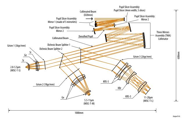
**Figure 3-16:** The MISC-T optical design. The three spectrometers are fed by a collimated beam that emerges from the tip-tilt sensor focal plane mask optics. The dimensions of the instrument in mm are indicated.
