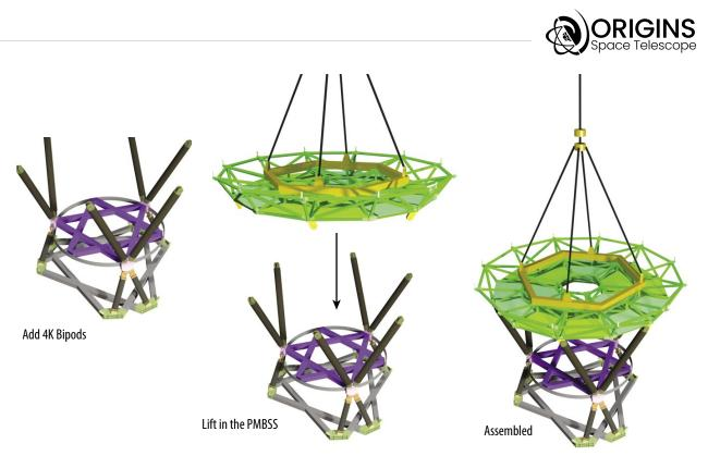
**Figure C-17:** The 4.5 K Bipods are supported until the PMBSS is installed.
