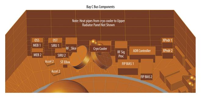
Figure C-11: There is plenty of space in each of the SBM bays for electrical boxes and other hardware. Here we show Bus Bay C.
