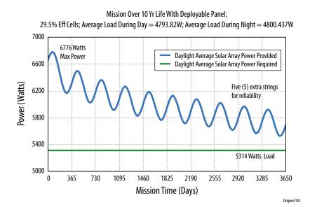
**Figure 2-37:** Solar Array Power and Load vs. Mission Time.
