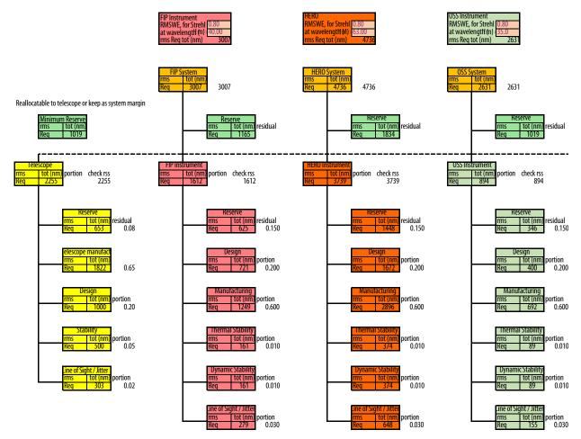
Figure C-46: Wavefront error budgets combining the allocations to the OSS, FIP, and HERO instruments with that of the telescope.
