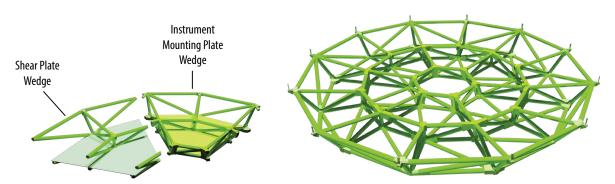
**Figure 2-29:** To optimize weight and strength, the PMBSS is a trussed design. The PMBSS is entirely beryllium to match the Coefficient of Thermal Expansion (CTE) of the Primary Mirror Segment Assembly. Three sets of PMBSS Wedge Subassemblies are fabricated and fastened together to comprise the whole PMBSS.
