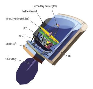
**Figure ES-8:** *Origins* builds on substantial heritage from *Spitzer* to minimize assembly, integration and testing, and deployment risks. A cutaway view shows the *Origins* instrument locations and major elements of the flight system.
