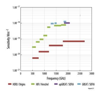
**Figure D-12:** HERO is more sensitive by an order of magnitude than any prior heterodyne instrument and has the widest frequency coverage of any previous instrument. (The sensitivity calculations for SOFIA assume a perfectly transparent atmosphere, which is not true close to the water lines.)
