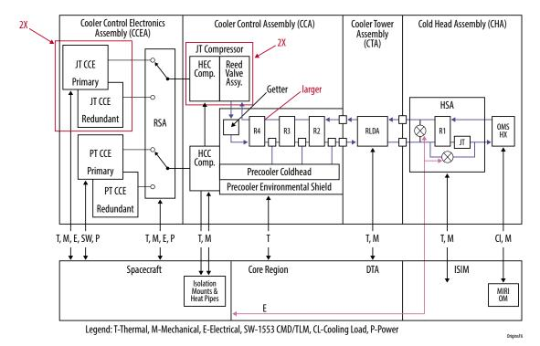
Figure F-5: 2 stage JTC compressor version of MIRI cooler modified for use on Origins
