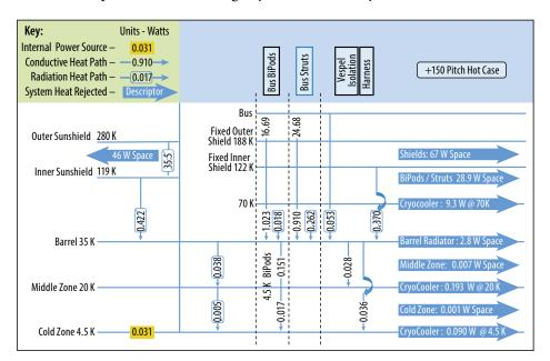
Figure 2-8: Origins Heat Flow Map of the CPM shows the multiple stages of cooling results in a reasonably small heat load to the cryocooler and radiative cooler stages
