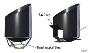
**Figure 2-18:** Barrel Support Struts support the Barrel and connect to the CPM Base, providing stiffness to the assembly. For clarity, the Bus Bipods are not shown. Doors for access to the instruments are notional. The doors, providing access to the instruments, harnesses, and cryocooler lines, may be hinged at the left and right rather than the top and bottom.
