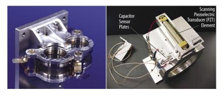
**Figure 3-12:** Heritage of scanning etalons for far-IR astrophysics. Left shows the dual etalon used in the Infrared Space Observatory (ISO) (credit Max Planck Institute for Extraterrestrial Physics, Garching).
