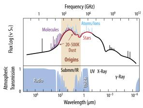
**Figure ES-2:** *Origins* studies the universe at a wavelength range that is inaccessible from the ground. Infrared photons between 2.8 and 588 µm in *Origins'* wavelength range capture emission from stars, molecules, dust, and ions/atoms, enabling a multi-pronged probe into key physical processes in galaxies.
