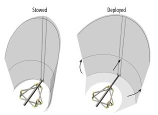
**Figure 2-20:** In the launch configuration, both shields are wrapped tightly around the Barrel. The simple linear deployment mechanism is attached to the Base and released on-orbit, allowing each shield to deploy. Outer Sunshield shown.
