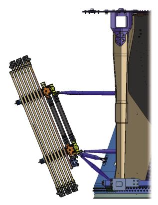
Figure F-8: Stowed 7 panel solar array on Webb Bus
