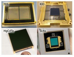
**Figure ES-10:** The robust Origins Technology Development Plan recommends parallel investment in four detector technologies. TES bolometers (HAWC+ array), KIDS (432-pixel device), HgCdTe arrays (JWST/NIRCam), and Si:As (JWST/MIRI).
