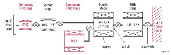
**Figure 3-29:** The FIP CADR provides continuous cooling at two stages: 50 mK (with 0.4 µK stability) and 0.7 K (with 0.1 mK stability), and deposits its heat at a 4.5 K heat sink.
