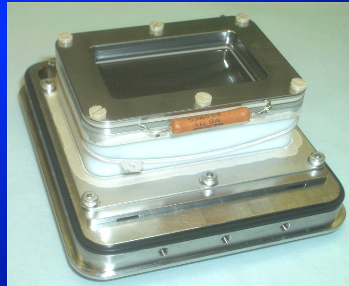
Rosetta Alice, Pluto Persi-ALICE, LRO-LAMP, JUNO-UVS. Delay line up to 2048 x 512, 50 – 180nm, CsI & KBr. High curved (7cm R) - spectrometers.
