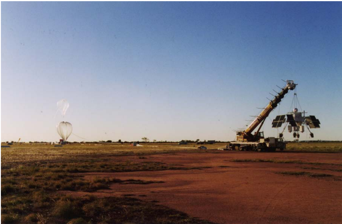
The NIGHTGLOW experiment in Alice Springs, Australia, prepares for a launch beneath a balloon that will lift the instrument above 99% of the atmosphere to measure ultraviolet light reflected by the Earth at night. Photo courtesy of the NIGHTGLOW team.
