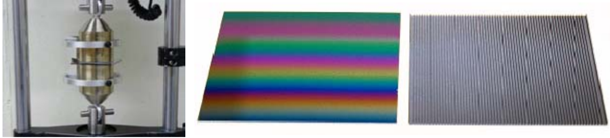
Figure 5 First pull tests performed on bonded plates (left). Wedged and ribbed silicon plates meeting the requirements of IXO (right).
