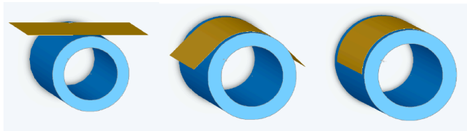
Mirror segment on a precisely figured mandrel
