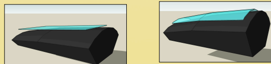
Fig. 4: Sketch of a possible configuration to slump a glass segment for X-ray optics.
