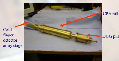
The Cooling parts (CPA and DGG) of the dADR
