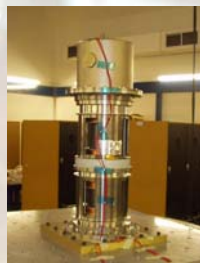
dADR mounted on the 4K stage of the ground test cryostat. Cooling to 4 K provided by a pulse tube cooler
