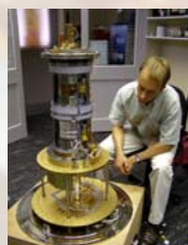
dADR mounted on the 4K stage of the ground test cryostat. Cooling to 4 K provided by a pulse tube cooler
