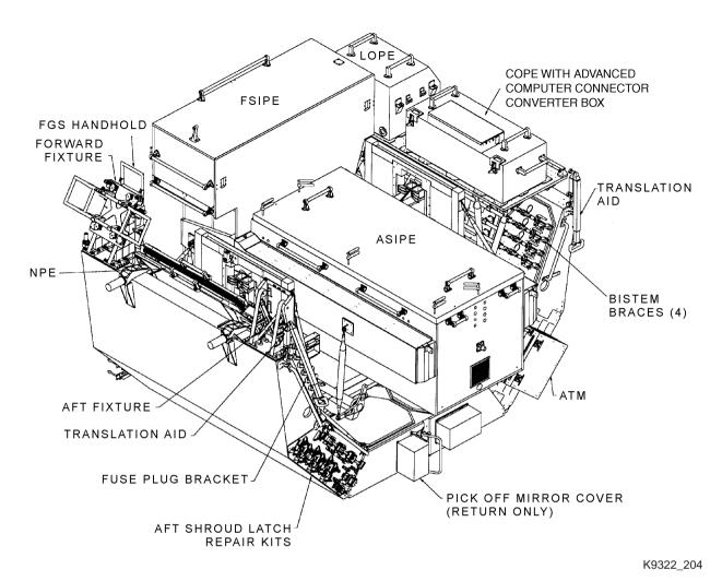
Fig. 2-4 Orbital Replacement Unit Carrier
