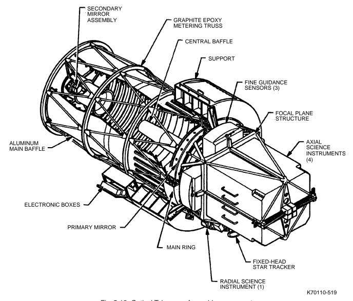
Fig. 5-19 Optical Telescope Assembly components
