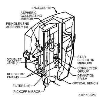
Fig. 5-26 Cutaway view of Fine Guidance Sensor
