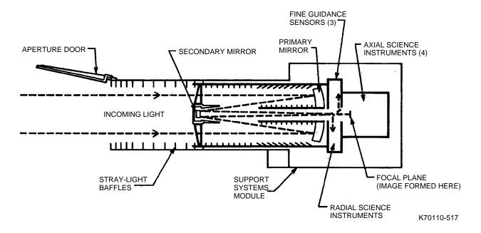
Fig. 5-17 Light path for the main Telescope
