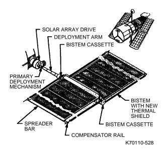
Fig. 5-28 Solar Array wing detail
