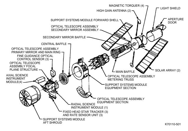
Fig. 5-1 Hubble Space Telescope – exploded view
