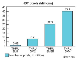
Fig. 7-5 Increase in onboard pixels
