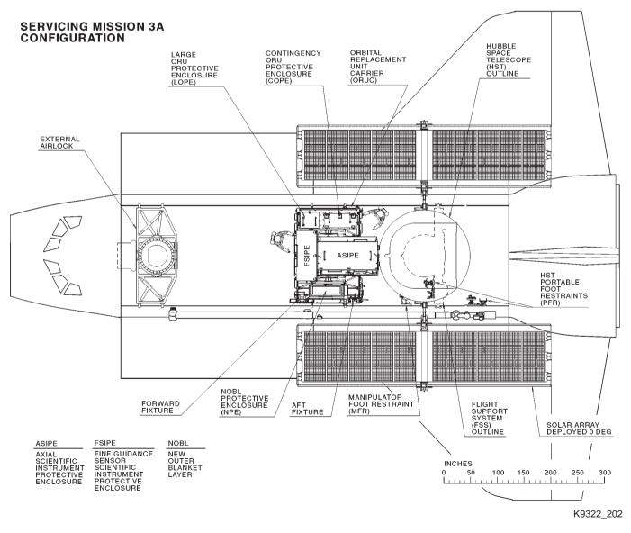
Fig. 2-2 Servicing Mission 3A Payload Bay configuration
