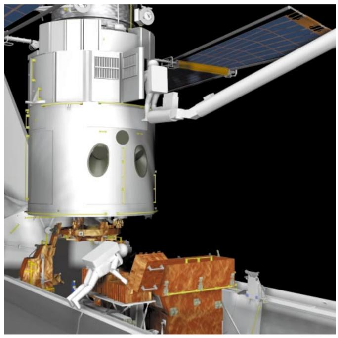
Fig. 2-9 Voltage/Temperature Improvement Kit installation
