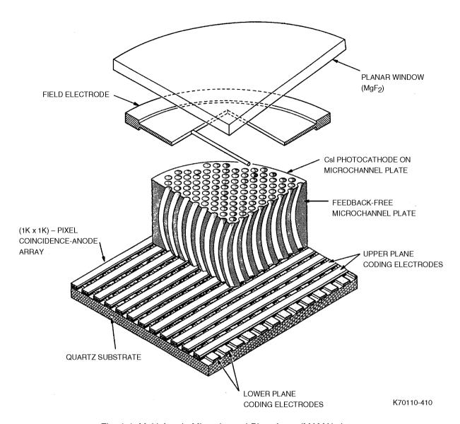
Fig. 4-4 Multi-Anode Microchannel Plate Array (MAMA) detector
