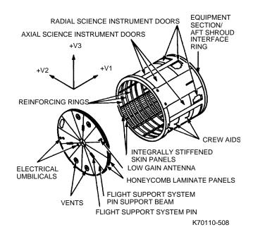
Fig. 5-8 Support Systems Module aft shroud and bulkhead
