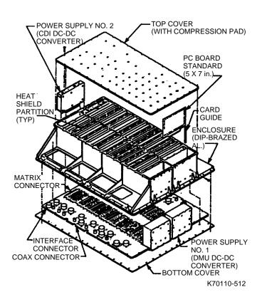
Fig. 5-12 Data Management Unit configuration
