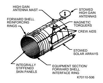
Fig. 5-6 Support Systems Module forward shell
