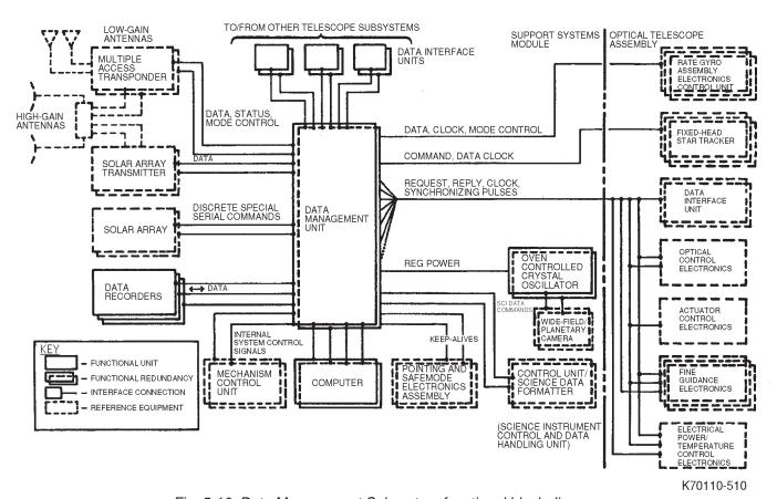
Fig. 5-10 Data Management Subsystem functional block diagram
