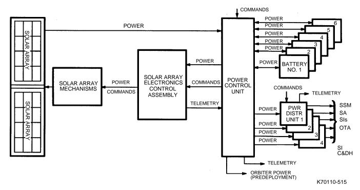
Fig. 5-15 Electrical Power Subsystem functional block diagram
