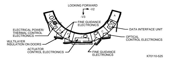
Fig. 5-25 Optical Telescope Assembly Equipment Section
