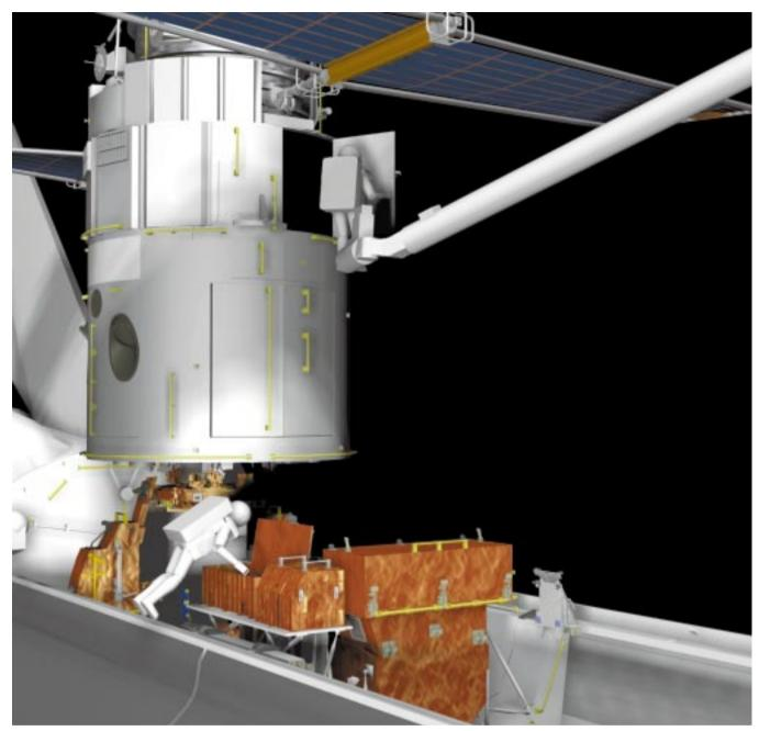
Fig. 2-11 S-Band Single Access Transmitter change-out
