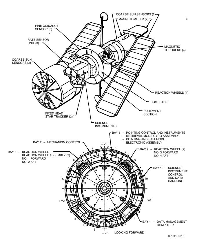
Fig. 5-13 Location of Pointing Control Subsystem equipment
