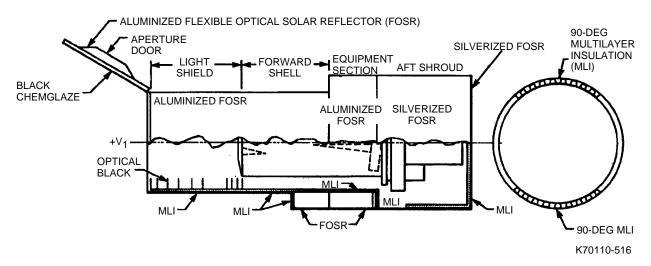
Fig. 5-16 Placement of thermal protection on Support Systems Module
