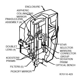
Fig. 4-12 Fine Guidance Sensor (FGS)
