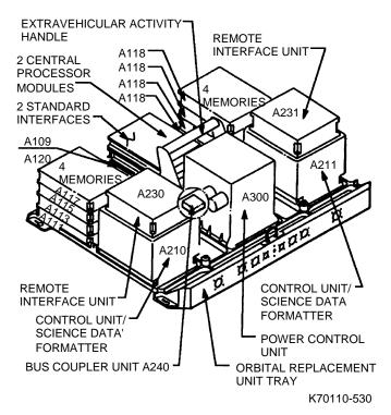
Fig. 5-30 Science Instrument Control and Data Handling unit
