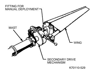
Fig. 5-29 Fitting for Solar Array manual deployment
