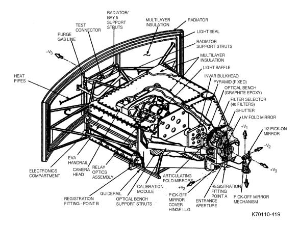
Fig. 4-8 Wide Field and Planetary Camera (WFPC) overall configuration
