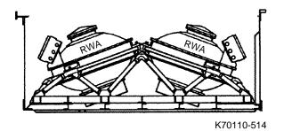
Fig. 5-14 Reaction Wheel Assembly
