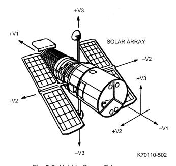
Fig. 5-2 Hubble Space Telescope axes
