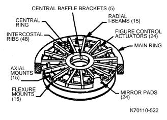
Fig. 5-22 Main ring and reaction plate
