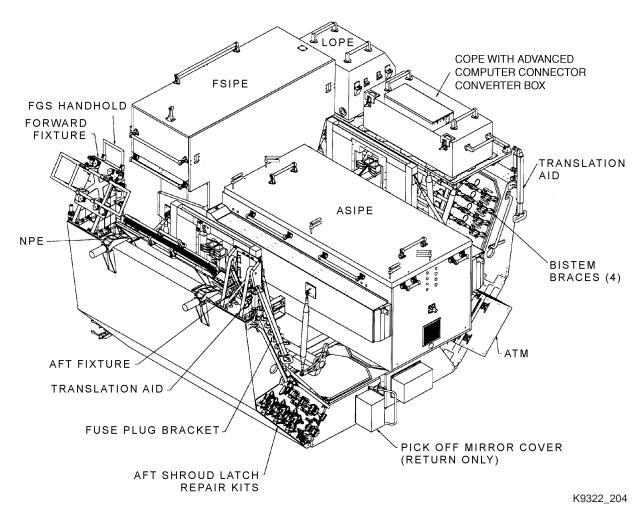
Fig. 5-35 Orbital Replacement Unit Carrier
