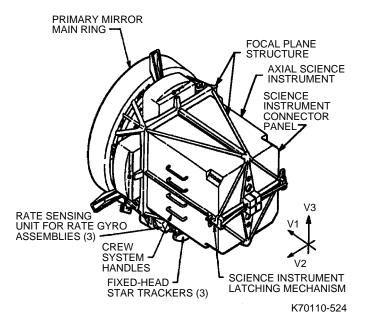
Fig. 5-24 Focal plane structure
