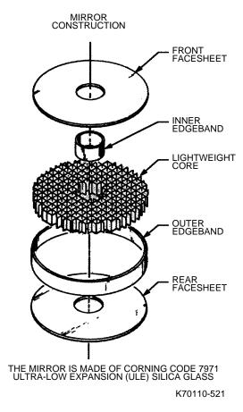
Fig. 5-21 Primary mirror construction
