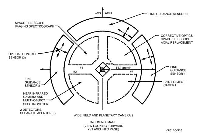
Fig. 5-18 Instrument/sensor field of view
