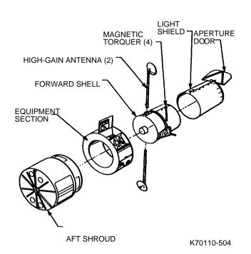
Fig. 5-4 Structural components of Support Systems Module
