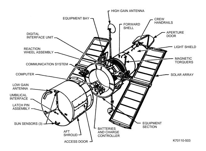
Fig. 5-3 Design features of Support Systems Module
