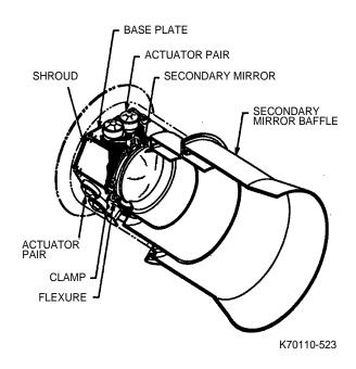
Fig. 5-23 Secondary mirror assembly
