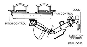
Fig. 5-36 Portable Foot Restraint
