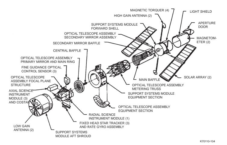
Fig. 1-4 HST exploded view
