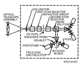
Fig. 5-27 Optical path of Fine Guidance Sensor
