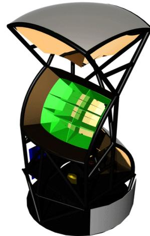
Figure 3: Cutaway view of 3 x 3 sub-telescope array for Right Telescope with active-passive collimator shields (green) each defining  $50^\circ \times 58^\circ$  FoV.
