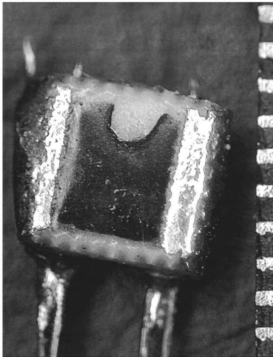
FIG. 1. RuO<sub>2</sub> surface mount resistor is shown. The marks on the scale are 0.01 in.
