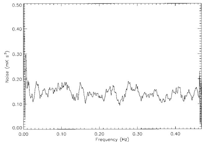
FIG. 7. Noise spectrum of one of the thermometers at 2.7 K.
