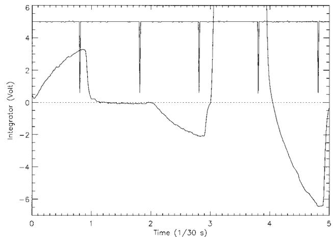
FIG. 4. Oscilloscope trace of five samples. The first sample is near 33 k $\Omega$ . The others are: 25 k $\Omega$  (the null point), 20 k $\Omega$ , open, and 10 k $\Omega$ , respectively. Also shown is the digitized command strobe.
