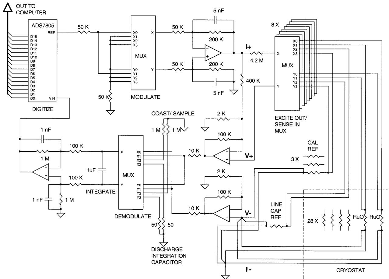
FIG. 2. Circuit diagram shows the major elements of the RuO<sub>2</sub> readout circuit. All of the multiplexers are CD4052 dual 4-to-1 analog multiplexers. The opamps are an LT1125 quad opamp. The integration capacitor is polypropylene for stability.
