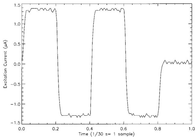
FIG. 3. Oscilloscope trace of the excitation current. The  $A \rightarrow D$  converter is activated at the beginning of the fifth phase.
