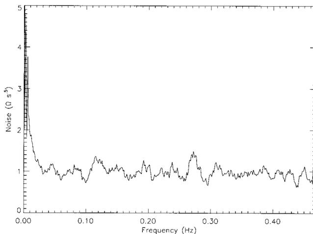
FIG. 6. Noise spectrum of one of the calibration resistors. This spectrum was taken between the relatively rare jumps of  $\sim 5$  counts. Each count corresponds to  $0.8 \Omega$ .
