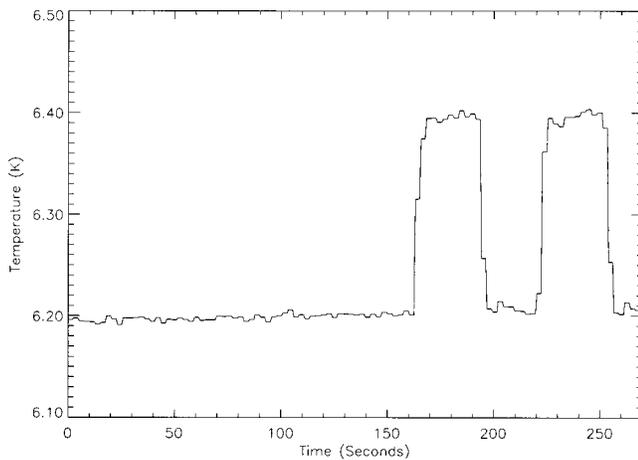
FIG. 5. 270 s of temperature data, demonstrating the control in switching between 6.2 and 6.4 K. The noise is higher at 6 K than at 2.7 K because of the  $dR/dT$  dependence on  $T$ . A careful look at the transitions shows an  $\sim 20$  s settling time.
