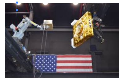
Final approach and capture box closed-loop demonstration
